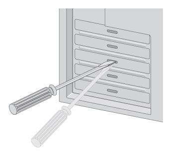
Figure 4. Removing the Faceplate from PCIe Slot
